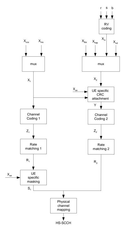
Figure 19: Coding chain for HS-SCCH type 1
